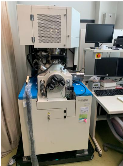
Fig. 3.7.(a) The FIB device SMI-3050 from Hitachi company. (b) The principle of the FIB process.
