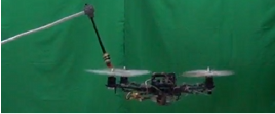
Figure 4.25: Collision experiment during drone hovering.
