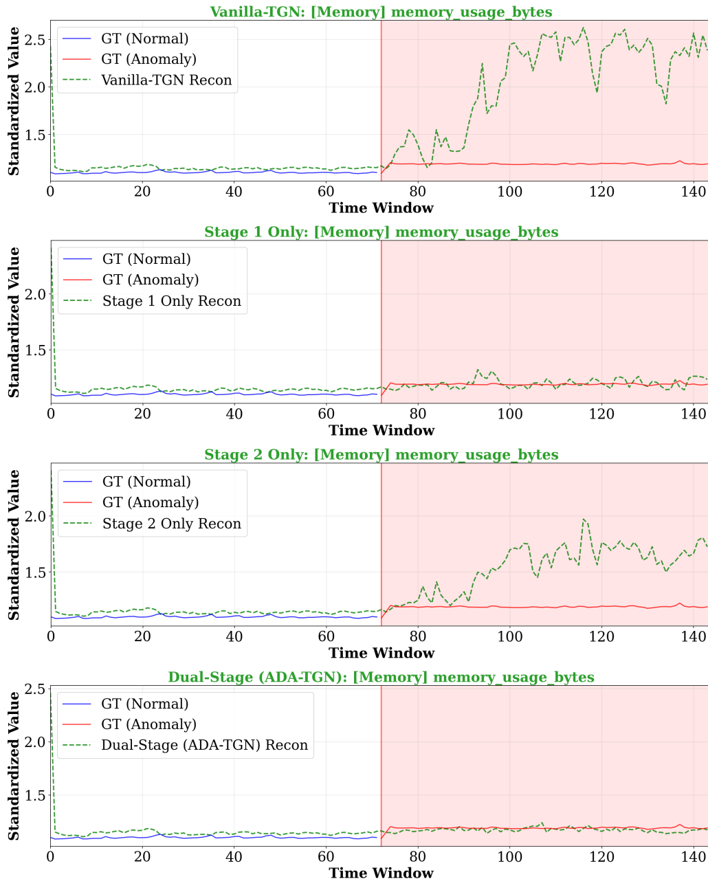
Figure 6.3: Reconstruction comparison for Memory (container_memory_usage_bytes). From top to bottom: Vanilla-TGN, Stage 1 Only, Stage 2 Only, Dual-Stage (ADA-TGN).
