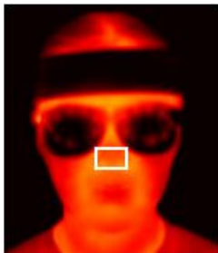
Figure 3.3: Extracted nasal region with privacy blur. Depicts the tracked nasal region used for thermal analysis while maintaining participant anonymity.
