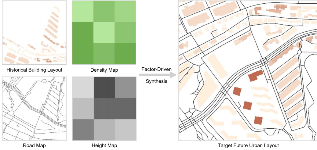
Figure 7.1: Overview of factor-driven urban layout modeling. The target urban layout is generated by incorporating multiple interdependent urban planning factors, such as building density, height map, road structure, and historical building patterns.
