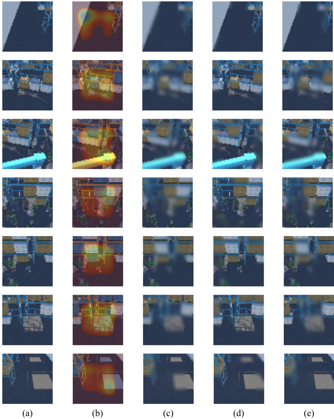
Figure A.1: Attention-guided input perturbation examples for simulation images. For each row, (a) the original input image, (b) the corresponding Grad-CAM attention map, (c) the image with blurring applied to high-attention regions, (d) the image with blurring applied to low-attention regions, and (e) the image with blurring applied to randomly selected regions of identical spatial extent are shown. This figure illustrates the perturbation design used for the interpretability analysis.
