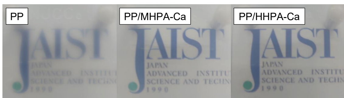
FIGURE 2.13 Photographs of injection-molded plates with 1 mm thickness.
