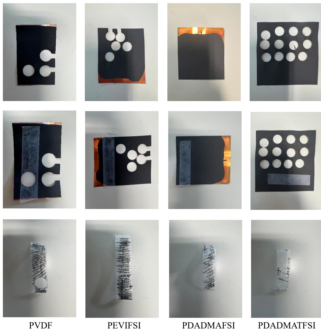
Figure 22. Scotch tape test to check the adherence of the electrode material to the current collector.
