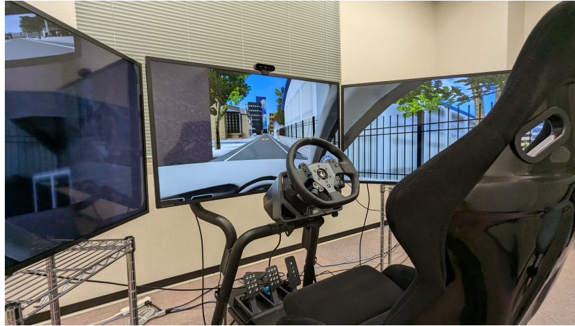
Figure 6.3: Driving simulator. The side displays offered peripheral views, and the subjects could check for oncoming cars or bicycles at the intersection.
