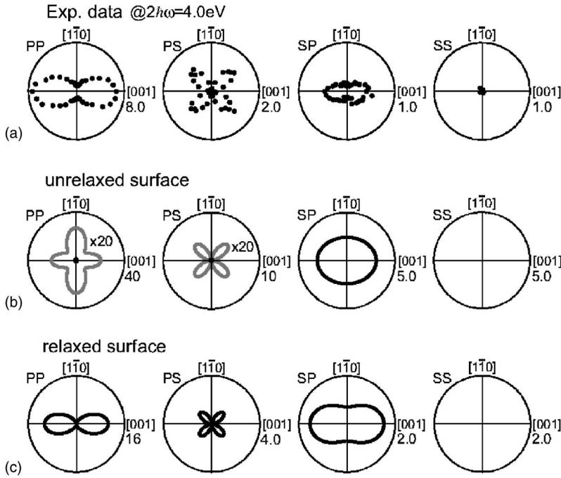
FIG. 6. SH intensity as a function of the sample rotation angle around the surface normal at the SH photon energy  $2\hbar\omega = 4.0$  eV: (a) experimental data of Ref. 15, (b) calculated patterns for unrelaxed surface, and (c) calculated patterns for relaxed surface. PP, PS, SP, and SS represent the polarization configurations of input and output fields. The units of the radial direction are arbitrary units.
