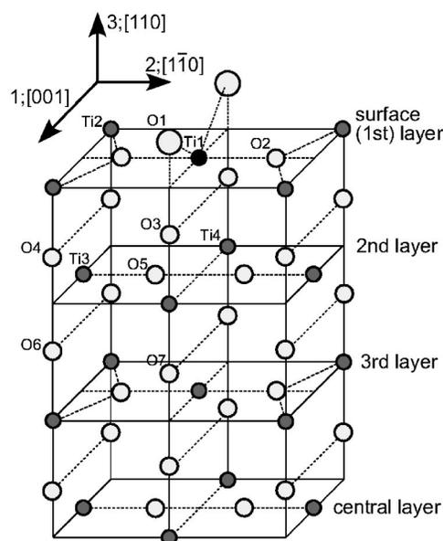
FIG. 1. Upper half of the rutile TiO<sub>2</sub>(110) slab for the calculation.
