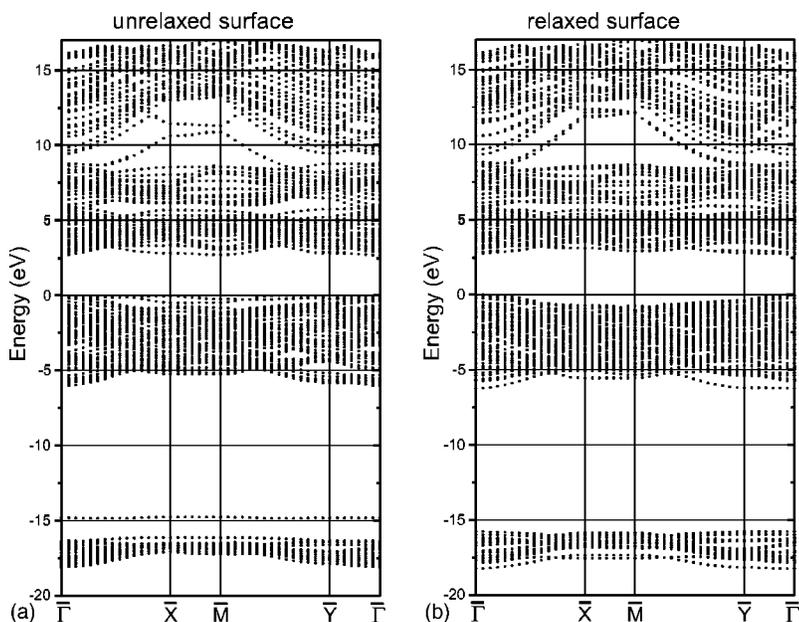
FIG. 2. Surface electronic band structures of (a) unrelaxed and (b) relaxed  $\text{TiO}_2(110)$  surfaces. The band gap is increased by a scissors operator with  $\Delta_{\text{QP}}=1.5$  eV.
