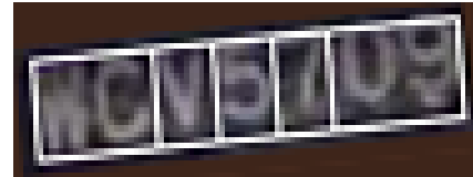
Fig. 2. Failed character segmentation resulting in some regions having more than one characters enclosed. This usually leads to recognition errors.
