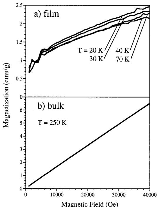
FIG. 3. The field dependence of magnetization at various temperatures for  $\text{La}_{0.4}\text{Ba}_{0.1}\text{Ca}_{0.5}\text{MnO}_{3-y}$  thin films (deposited with the oxygen pressure of 70 mTorr) and bulk.
