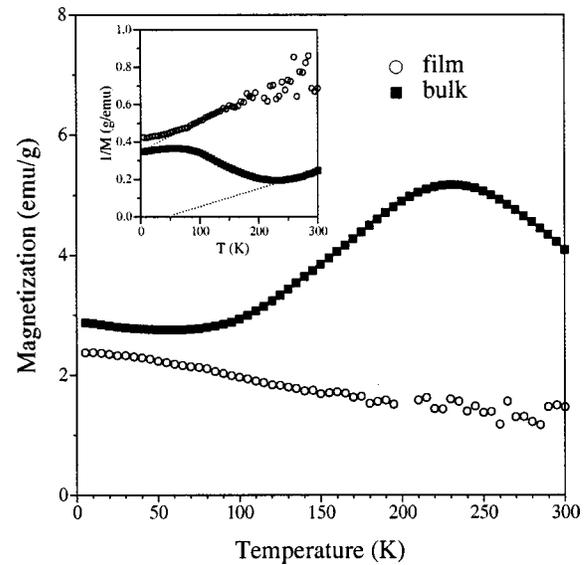
FIG. 2. The temperature dependence of magnetization at 3 T for  $\text{La}_{0.4}\text{Ba}_{0.1}\text{Ca}_{0.5}\text{MnO}_{3-y}$  thin films (deposited with an oxygen pressure of 70 mTorr) and bulk. The inset shows  $1/M$  vs  $T$ , and the interceptions of the dashed lines and  $T$  axis indicate  $\theta$ .
