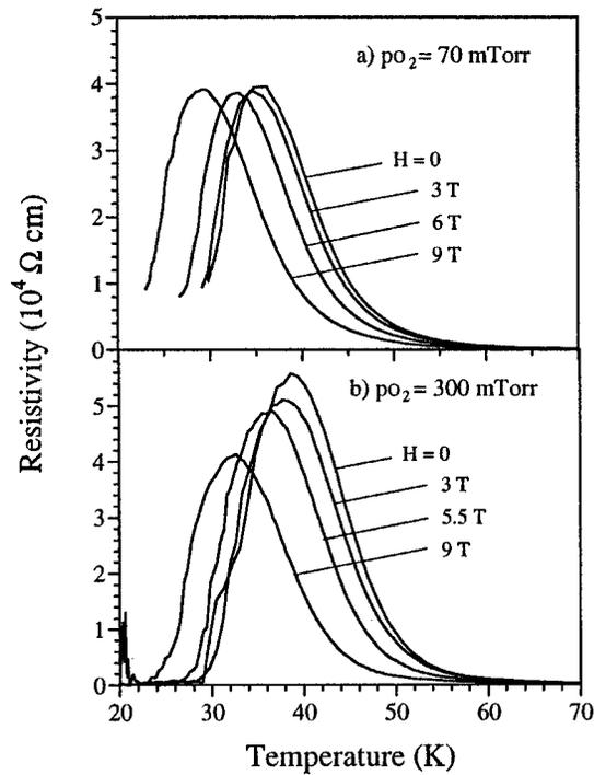
FIG. 1. The temperature dependence of resistivity at various fields for  $\text{La}_{0.4}\text{Ba}_{0.1}\text{Ca}_{0.5}\text{MnO}_{3-y}$  thin films deposited with the oxygen pressure of (a) 70 mTorr and (b) 300 mTorr.
