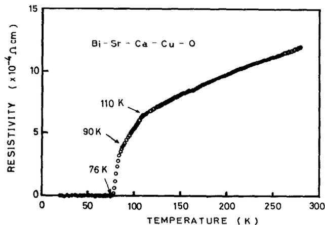
FIG. 3. Resistivity vs temperature for an as-grown Bi-Sr-Ca-Cu-O film deposited on a (100)MgO substrate.
