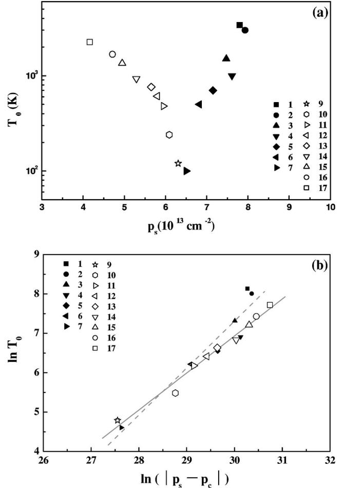
FIG. 5. (a) Plots of the scaling parameter  $T_0$  as a function of the hole concentration  $p_s$ . (b) Plots of the scaling parameter  $T_0$  as a function of  $|p_s - p_c|$  on a log-log scale where  $p_c$  is the critical hole concentration.
