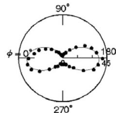
Fig. 1 SH intensity from Au nanowires as a function of the sample rotation angle  $\phi$  for *p*-in/*p*-out polarization combination. When  $\phi=0^\circ$ , the incident plane is parallel to the nanowire axes. The photon energy of the excitation field is  $\hbar\omega=1.17\text{eV}$ .
