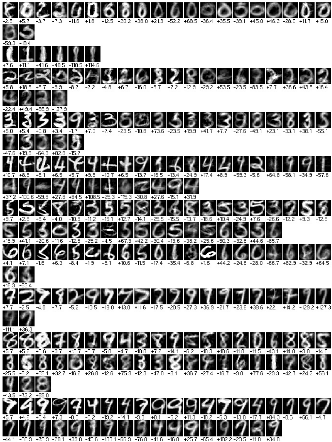
Figure 3.7: Display of all vectors in simplified solutions. The original 10 classifiers trained with polynomial kernel of degree three and the cost C = 10 consist of 4538 SVs and produce 88 errors (on 2007 testing data). The simplified 10 classifiers consist of 270 vectors and produce 95 errors. The number below each image indicates the new weight of a reduced vector.
