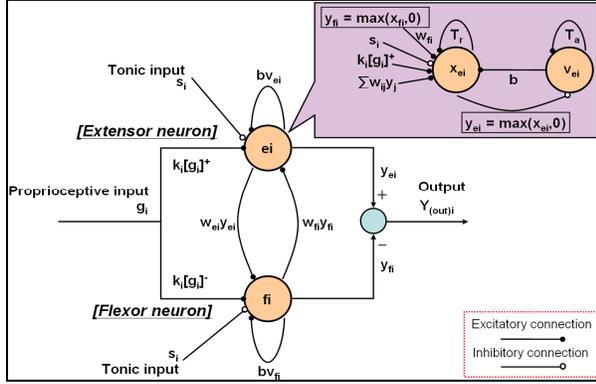
Fig. 1. Schematic diagram of Matsuoka Neural Oscillator
