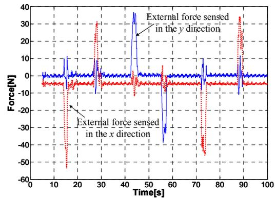
Fig. 8. The external forces measured by the force sensor in the  $x$  and  $y$  direction
