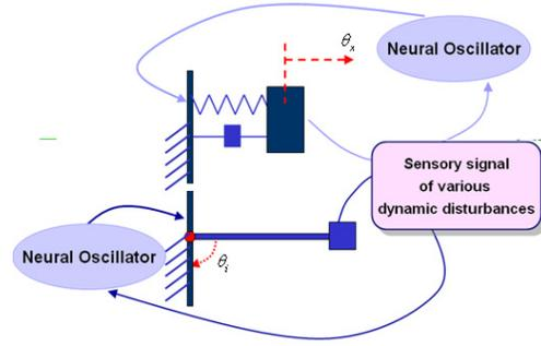
Fig. 2. Mechanical system coupled to the neural oscillator
