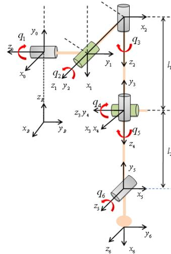
Fig. 6. Kinematic parameters of the robot arm
