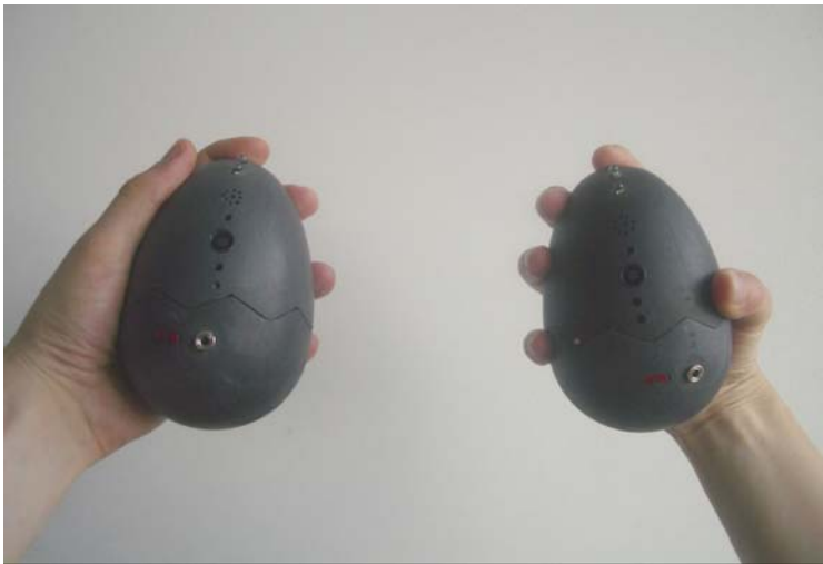
図5.5 Two “Mobile Feelings” interface devices which enable users to wirelessly transmit and receive each others’ heartbeat and breath.
