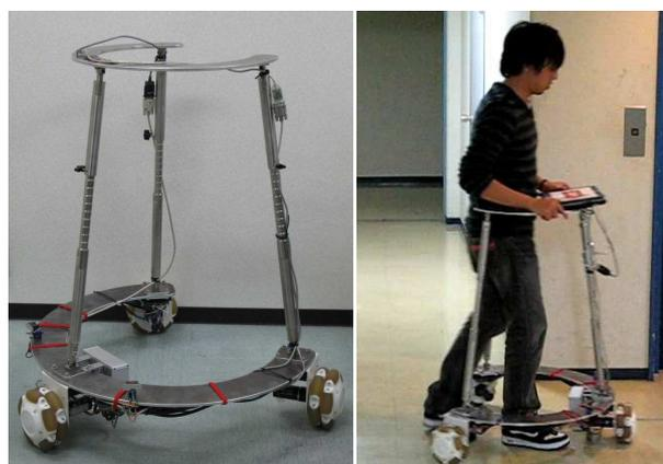
Fig. 1 JAIST active robotic walker (JARoW) prototype
