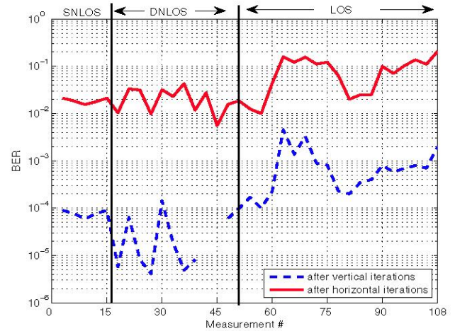
Fig.5. BER for the CST SC-MMSE after the last VI (dashed line) and after the last HI as the SNR=3dB.
