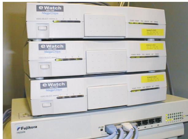
Figure 8: Multi-media broadcasting server and dual-speed Ethernet hub.
