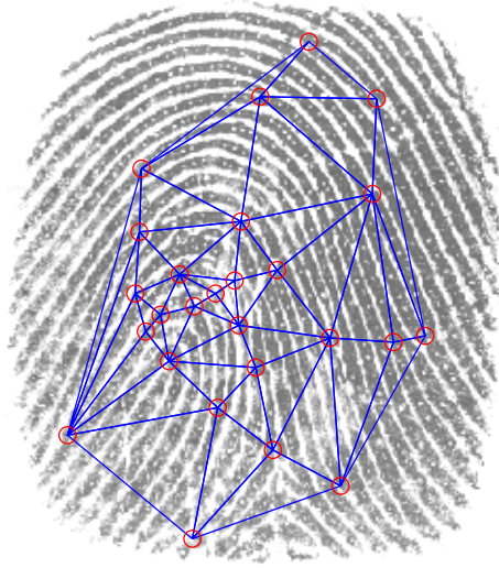
Figure 7.3: The Delaunay triangulation of minutiae.
